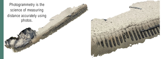
Faye shipwreck GIS map created using the total station collected points and photogrammetry.
