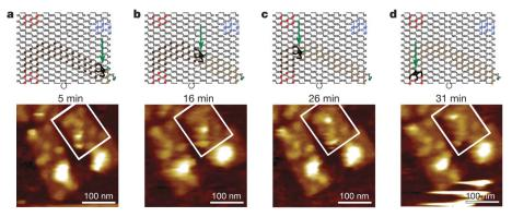
**Figure 3** | **AFM movie of spider movement. a**–**d**, Schematics and AFM images of the spider moving along the EABD track 5 min (**a**), 16 min (**b**), 26 min (**c**) and 31 min (**d**) after TRIGGER was added. AFM images are 300 nm × 300 nm and the scale bars are 100 nm.
