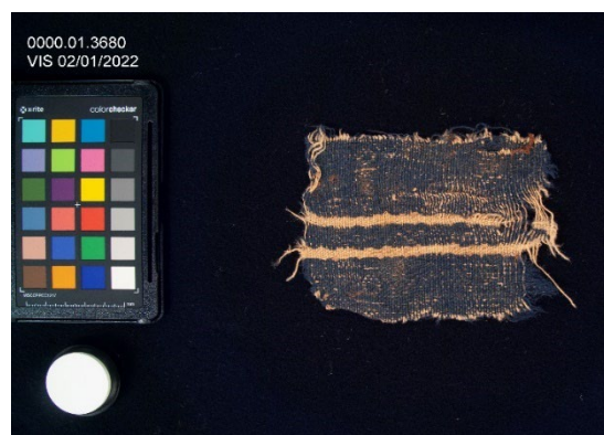
Figure 2. An example of a labeled visible light image with color checker and reflectance standard in the shot
