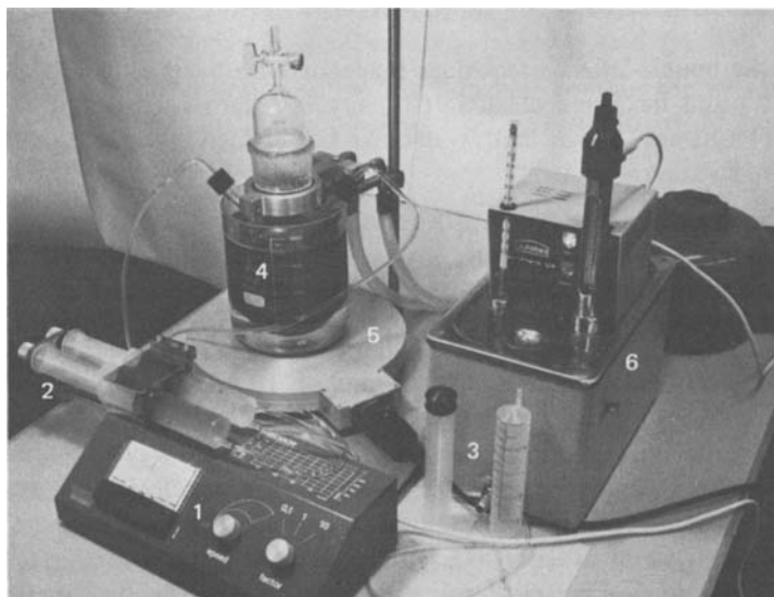
Fig. 2. Crystal-growth unit for rare earth hexacyanoferrates(III): (1) micro-pump, (2) syringes, (3) details of a syringe, (4) crystal-growth vessel surrounded by a copper-coil heat exchanger (connected with (6)), (5) heater for heating the oil in the outer vessel to slightly below the desired growth temperature, (6) thermostating unit for the heat exchanger.
