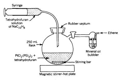
Fig. 1. Apparatus for platinum(0) complexes.
