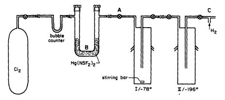
Fig. 1. Apparatus for synthesis of CINSF<sub>2</sub>.
