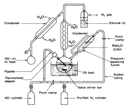
Fig. 1. Apparatus for syntheses of bis(alkylammonium)tetrachlorochromate(II) compounds.
