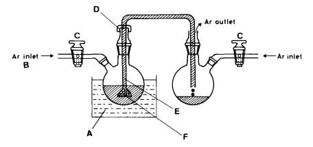
Fig. 2. Inverse filtration at low temperature. A, cooling bath, Dry lce/acetone; B, argon pressure maintained at 10-20 torr above atmospheric pressure; C, three-way stopcock; D, rubber cap; E, polyethylene tube, 3 mm, widened to 10 mm at one end; F, filter wad, cotton or glass wool.
