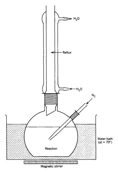
Fig. 1. Apparatus for preparation of dinitrogen complexes.
