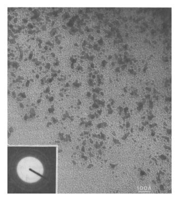
Fig. 1. Transmission electron micrograph of platinum microcrystals, with the corresponding Pt diffraction rings in the lower left corner. The granular background is the amorphous carbon film support.
