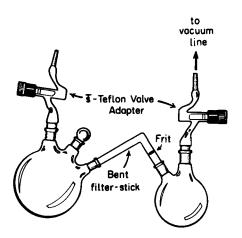
Fig. 1. Bent filter-stick filtration apparatus.
