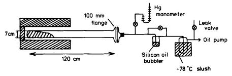
Fig. 1. Setup for the synthesis of  $Hg(CF_3)_2$ .
