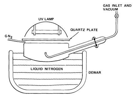
Fig. 1. Apparatus for synthesis of  $[NF_4][BF_4]$ .
