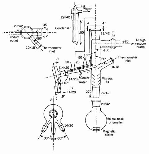
Fig. 1. Short-path distillation apparatus.
