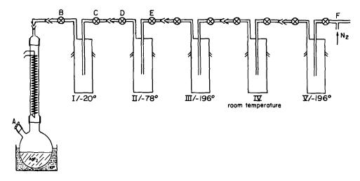
Fig. 1. Apparatus for the synthesis of  $NSF_3$  and for separation of products by trap-totrap fractionation.
