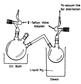
Fig. 1. Apparatus for isolation of alkyl metal compound by distillation.
