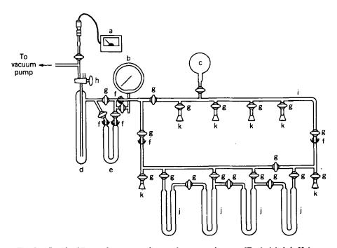
Fig. 1. Standard Pyrex glass vacuum line: a, thermocouple gauge [Fredericks]; b, Heise-Bourdon tube gauge [Dresser]; c, reservoir, 500 mL; d, removable cold trap; e, removable U-trap; f, 18/9 ball-and-socket joint; g, 2-mm Pyrex high-vacuum stopcock [Kontes]; h, three-way high-vacuum stopcock; i, Pyrex glass manifold, 10–12-mm diam; j, Pyrex glass traps to fit into a standard Dewar flask; k, 10/30 outer joint.
