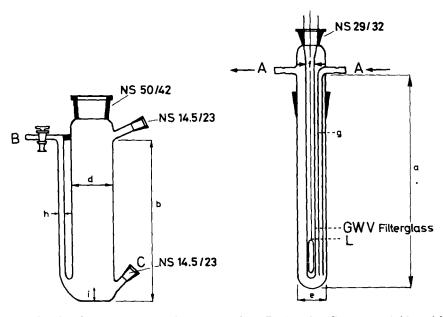
Fig. 1. Irradiation apparatus. A, water cooling; B, Ar inlet; C, septum (rubber) for withdrawing IR samples;  $\mathbf{L} = high$ -pressure mercury lamp (Philips HPK, 125-W), used in connection with a Philips VG1/HP 125-W power supply converter unit. Dimensions (in mm):  $\mathbf{a} = 400$ ,  $\mathbf{b} = 240$ ,  $\mathbf{d} = 70$ ,  $\mathbf{e} = 44$ ,  $\mathbf{f} = 28$ ,  $\mathbf{g} = 6$ ,  $\mathbf{h} = 10$ ,  $\mathbf{i} = 10$ .
