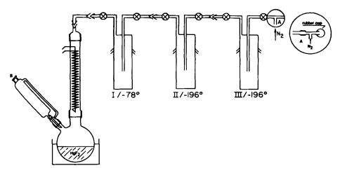
Fig. 2. Apparatus for the synthesis of  $Hg(NSF_2)_2$ .
