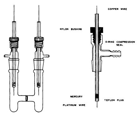
Fig. 1. Electrochemical cell and inset. Reference 7.
