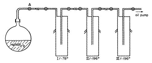
Fig. 3. Apparatus for thermal decomposition of  $Hg(NSF_2)_2$  to give NSF.
