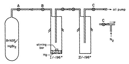
Fig. 2. Apparatus for synthesis of BrNSF<sub>2</sub>.
