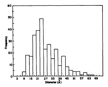
Fig. 2. Histogram of the diameters of the platinum microcrystals. The sample population is 300.
