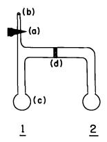
Fig. 1. Two-bulbed glass reaction vessel. (a) Teflon-stemmed Pyrex valve [Kontes]; (b)  $\frac{1}{4}$ -in. o.d. glass tubing joined to the manifold via a Hoke or Whitey (1KS4) [Whitey Tool] metal valve and Swagelok Teflon compression fittings [Crawford Fitting]; (c) thickwalled glass bulbs (8–15 mL); and (d) coarse sintered glass frit.
