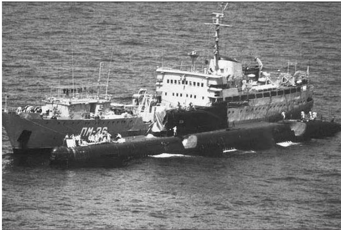
A Juliett-class submarine being repaired at sea
